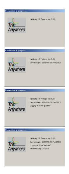
These screens show the stages of the login process. First the protocol is initialized, the client then contacts the server, the server logs you on, and then you are authenticated.
