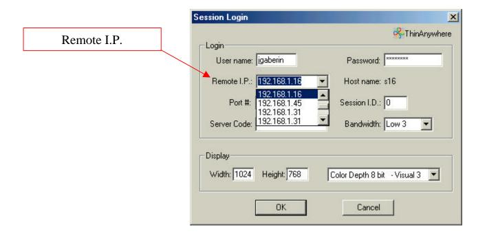
The **Remote I.P.** field of the Session Login screen displays the default servers that are in the ixlc.ini file. You may also type in an I.P. address. To edit the ixlc.ini file click on "Start"/"Program Files"/" Mercury International Tech" and then click the link for "View INI file".
