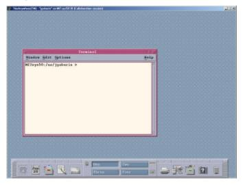
If the Originator accepts the request to collaborate then the Collaborator's client opens a window and connects to the same X session as the Originator's allowing both users to see and interact with the same screen/application.
